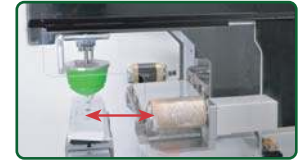
Pad in/out stroke for max. throat depth
