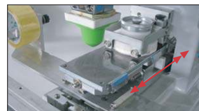
Platform in / out movement (Pad clean underneath)
