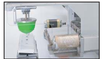
Pad in/out stroke for max. throat depth
