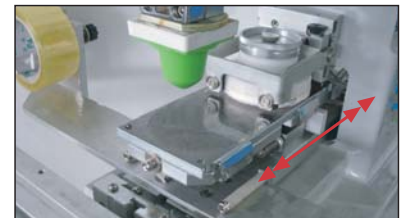
Platform in / out movement (Pad clean underneath)
