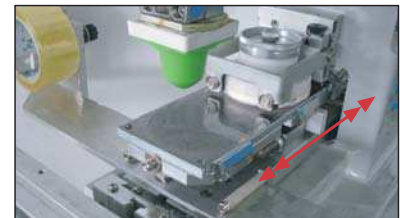
Platform in / out movement (Pad clean underneath)
