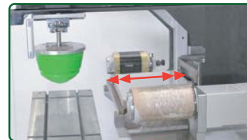
Platform in / out movement & pad clean underneath design for max. product size
