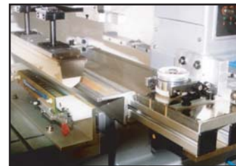
Side way ink cup for long image printing (SCMIC)
