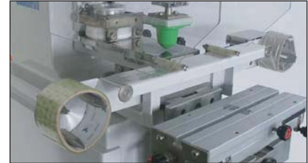
Automatic pad clean between work table and printing platform
